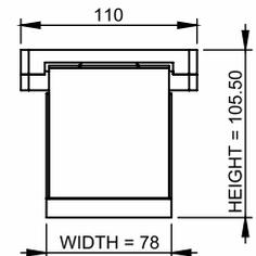
Ø 7 X 9.5L THRU SLOT X 4NO.S MOUNTING SLOTS WITH Ø 11 COUNTER
